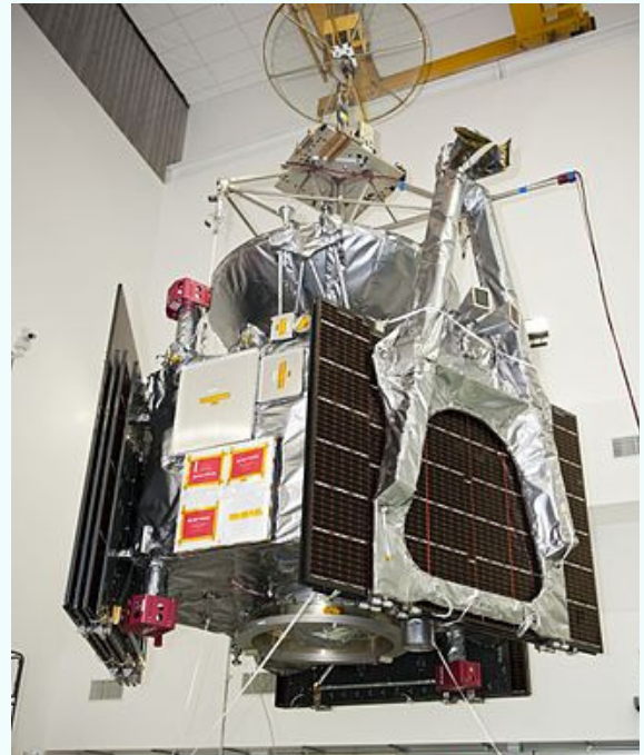
Microwave Radiometer (MWR) is an instrument on the Juno orbiter sent to planet Jupiter.
